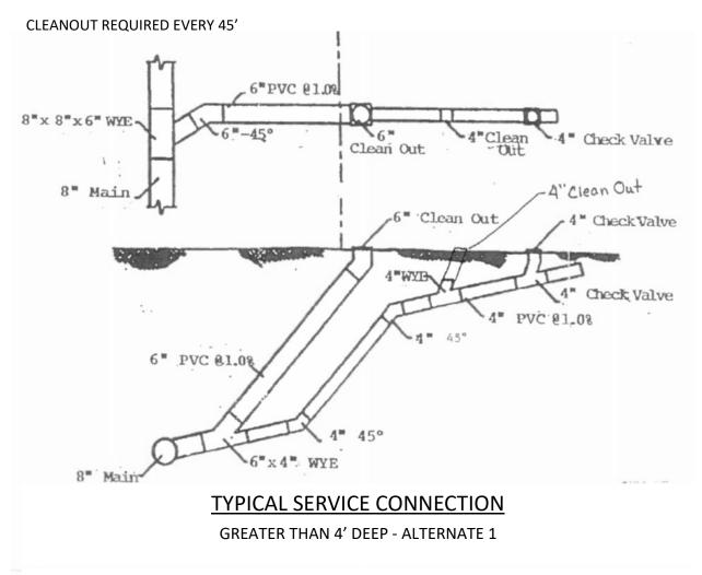
Boxes are **required** on 6" cleanout. Boxes are **optional** on 4" cleanout and 4" check valve.
