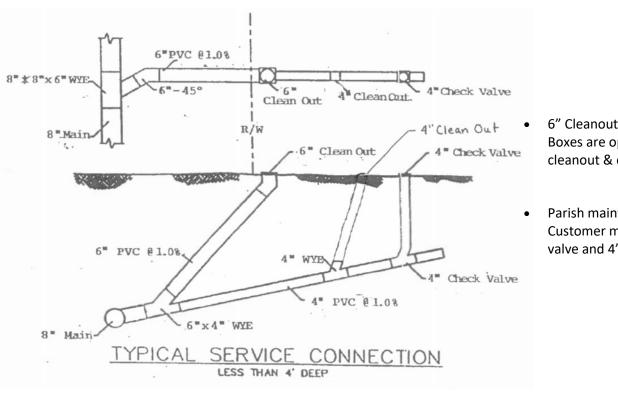
6" Cleanout = box REQUIRED! Boxes are optional on 4" cleanout & check valve.
